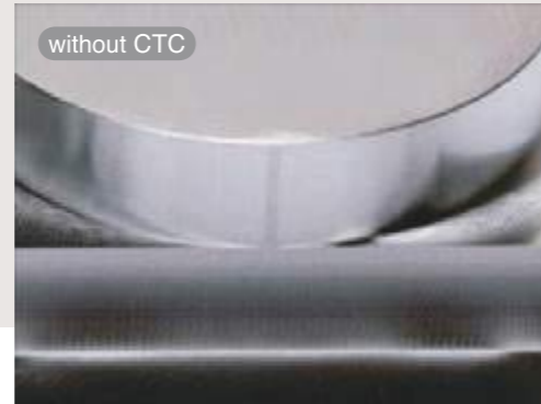
CTC compensation of position errors at the tool centre point generated by acceleration forces.
