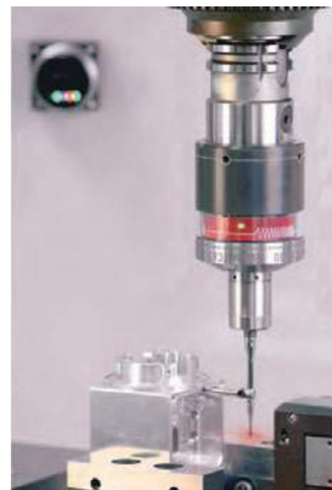
▲ Wireless workpiece measurement, no cover issue
