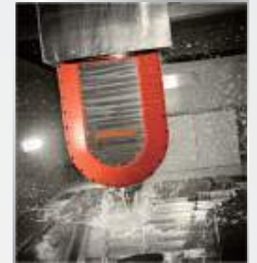
Multiple choose of 2 axis milling head and spindle HSK-A63 24000rpm & HSK-A100 12000rpm
