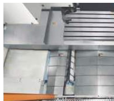
Bottom guarding flush + Screw chip removers
