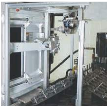
Work feeder (multiple pallets) and Turnover station
