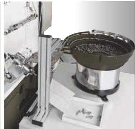
Work feeder (vibrator)
