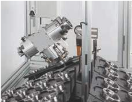
Work feeder (flexible)
