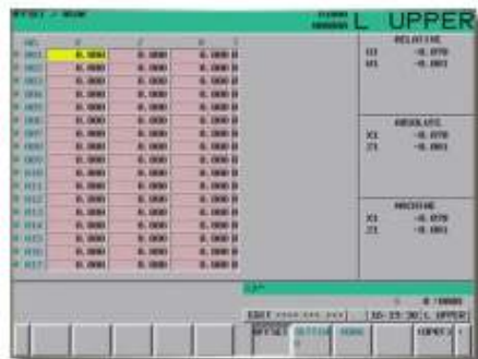
Tool offset setting & display 10.4"
