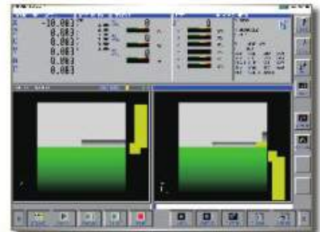
Cutting paths on 2 parts in MGI
